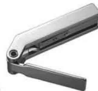
321.120 1 Tension Device, articulated Span 20mm, can also be used as a distractor. Colour scale: yellow up to 500N, green up to 1000N, red above 1000N.
